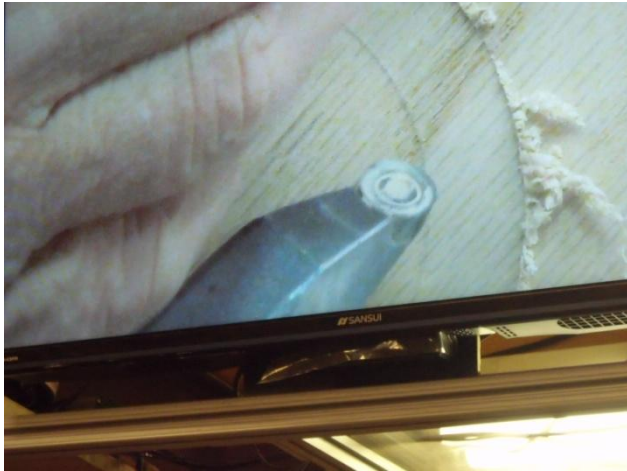
Shear scraping with the Hunter carbide tool.
