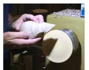
Sanding is done with a disk mounted on the lathe. Use a foam pad
