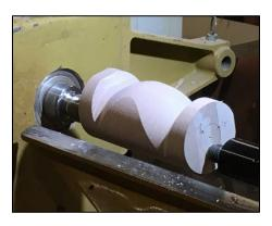
Eric uses the skew chisel for his turning, but noted that the spindle gouge can be used as well, and he demonstrated this. The spindle gouge, however, isn't able to get into the deep recesses that the skew can. Also note that this turning sometimes requires a lot of 'overhang' for the tool so you should use a fairly hefty tool. A 3/8" spindle gouge is too light.
