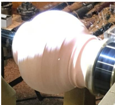
Roughing to shape, Leave extra material at the bottom until final shaping.
