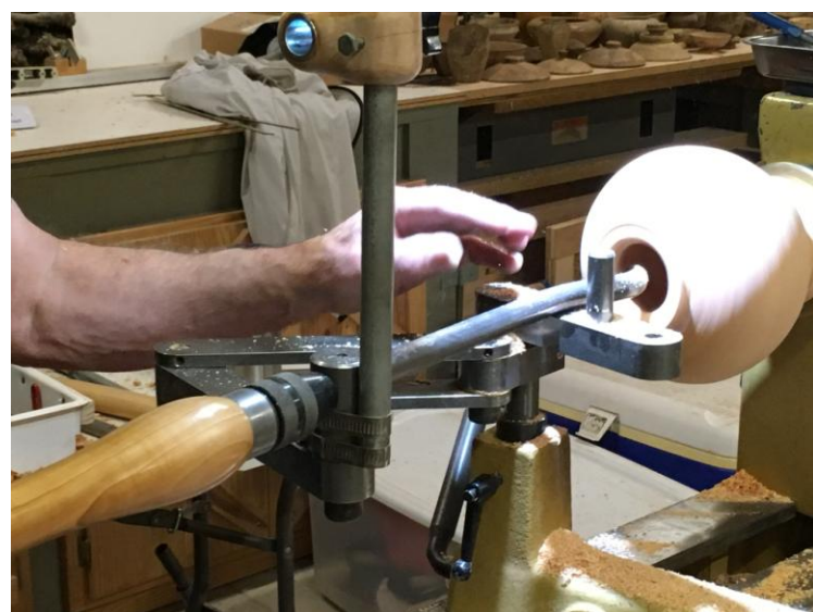
The last system he used was the Trent Bosch hollowing tool and jig.
