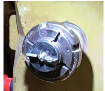
Two spur drive works well for wet wood.
